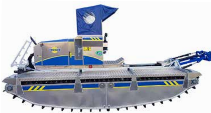
The movable driver's cab is hydraulically adjusted and works as counterweight during heavy lifts in water.
